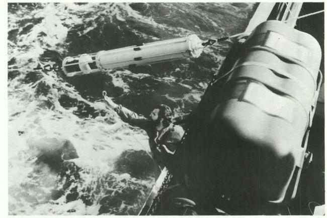
UP FROM THE DEPTHS, 6 km below, a current meter is hauled aboard the *Moana Wave*, the University of Hawaii's research vessel. The meter holds one of the first long-term (more than a month) records of ocean currents from water that deep. Unit was released from its anchor via radio command after 9 months of data collection.
